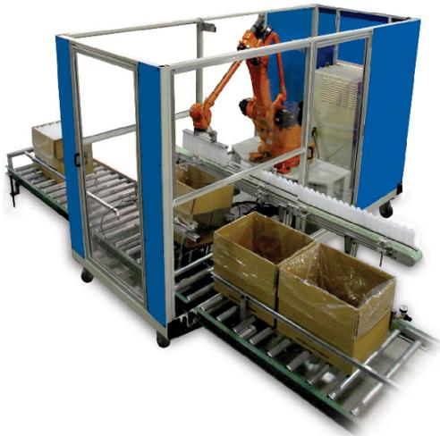
This system consists of a fully Articulated Six Axis Robot mounted on a structural sub frame complete with In-feed Product Conveyor, Box In-feed and Exit roller conveyor and safety guards.
